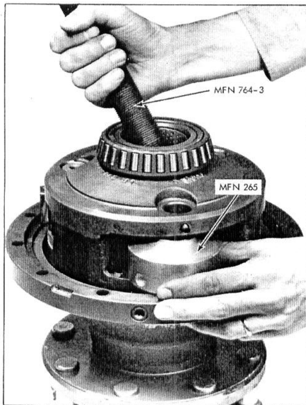
Fig. 29 - Special Tool MFN 265 and MFN 764-3 Installation or Removal
