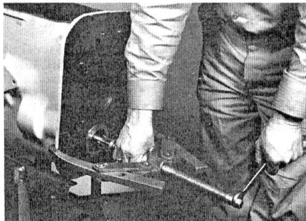
Fig. 5 - Pushing Countershaft Out of Rear Bearing
