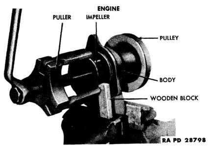
Figure 16 — Removing Water Pump Impeller, Using Puller (41-P-2912)
