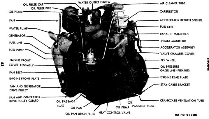
Figure 41 - Left Front View of Engine
