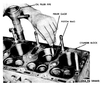
Figure 23 - Measuring Piston Ring End Gap with Feeler Gage
