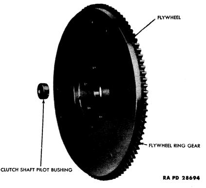
Figure 31 — Flywheel Ring Gear and Pilot Bushing
