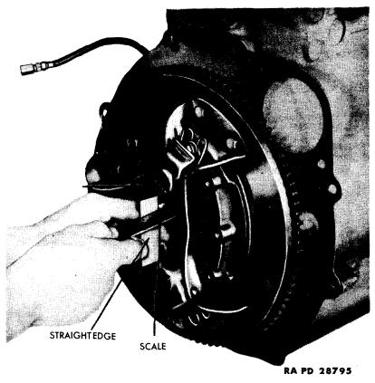
Figure 52 — Adjusting Pressure Plate
