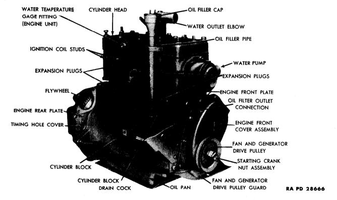
Figure 9 - Three-quarter Right Front View of Stripped Engine
