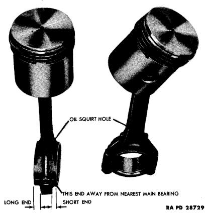
Figure 36 — Position of Connecting Rod Off-set and Oil Squirt Hole When Installed in Engine
