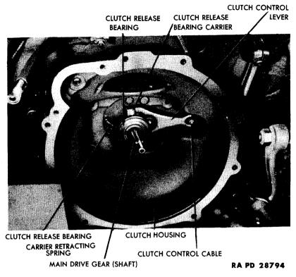
Figure 44 - Clutch Housing Installed in Vehicle
