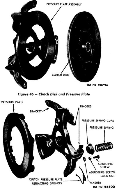
Figure 47 — Pressure Plate Disassembled
