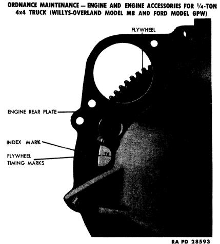
Figure 38 — Flywheel Timing Marks, T.C. (Top Center)
