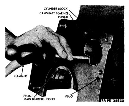
Figure 14 - Driving Camshaft Bearing from Cylinder Block
