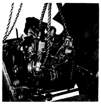
Figure 7 - Lifting Engine from Vehicle
