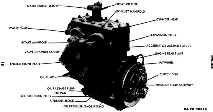
Figure 8 – Three-quarter Left Rear View of Stripped Engine
