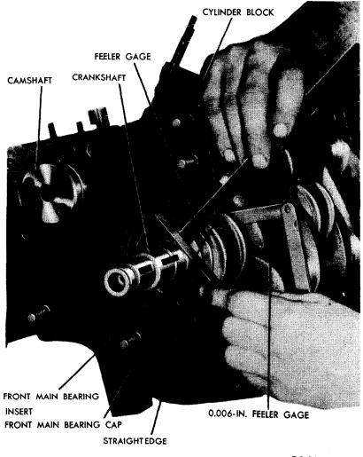
RA PD 28695 Figure 34 — Measuring Crankshaft End Play
