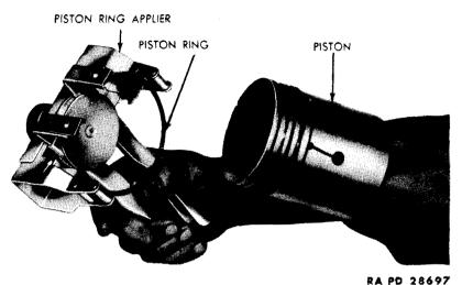
Figure 24 – Installing Piston Ring on Piston, Using Applier (41-A-329-500)
