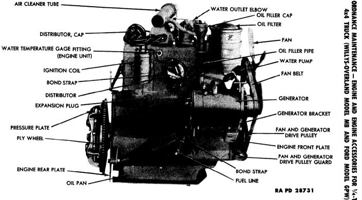
Figure 43 - Right Side View of Engine
