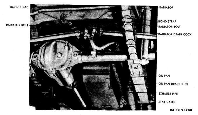
Figure 4 – Underside View of Engine Installed in Vehicle
