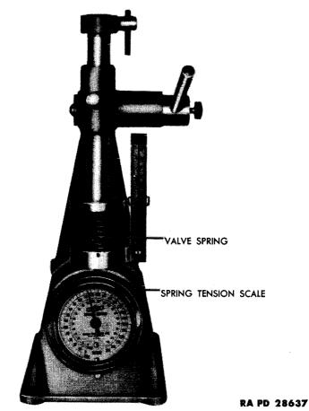
Figure 27 — Checking Tension of Valve Spring, Using Tester (41-T-1600)
