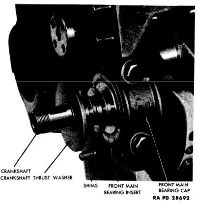
Figure 35 — Shims in Place on Crankshaft
