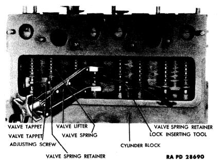
Figure 32 — Installing Valve Spring Retainer Locks, Using Lifter (41-L-1410) and Replacer (41-R-2398)
