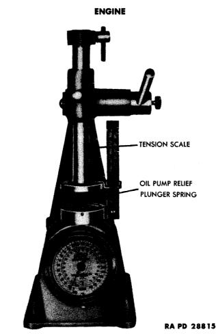
Figure 29 — Checking Oil Pump Relief Valve Spring Tension, Using Tester (41-T-1600)
