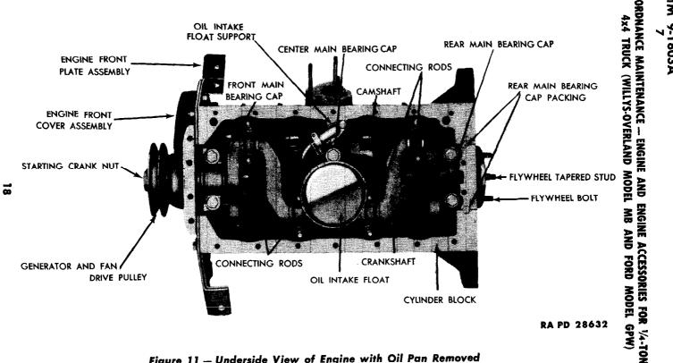
Figure 11 – Underside View of Engine with Oil Pan Removed
