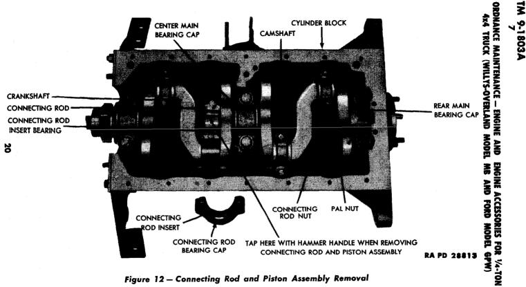
Figure 12 – Connecting Rod and Piston Assembly Removal
