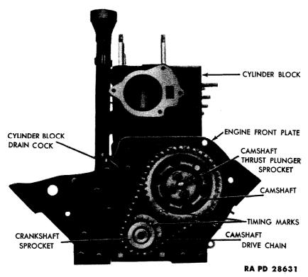
Figure 40 - Camshaft Timing Marks
