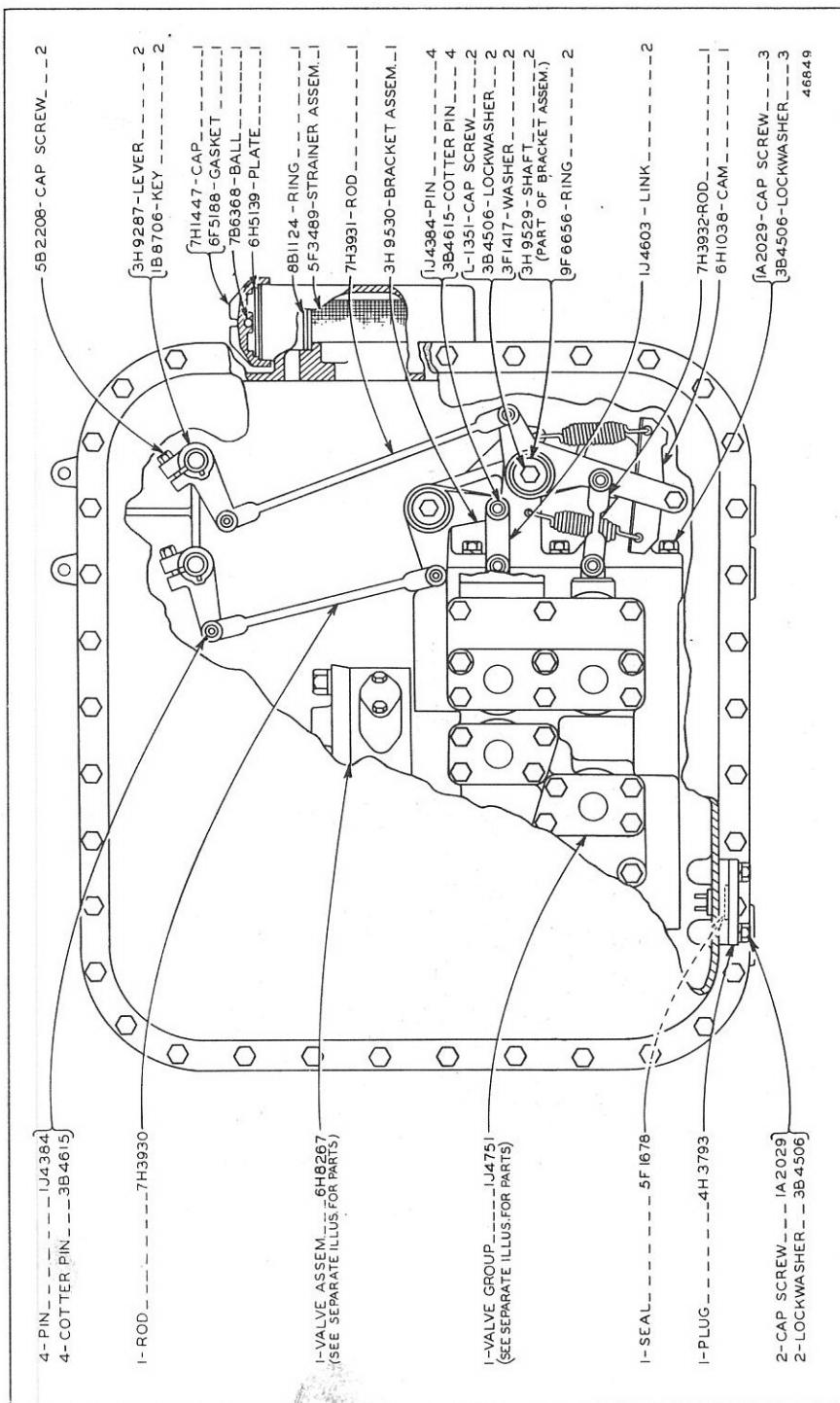
HYDRAULIC VALVE AND TANK—Front View
