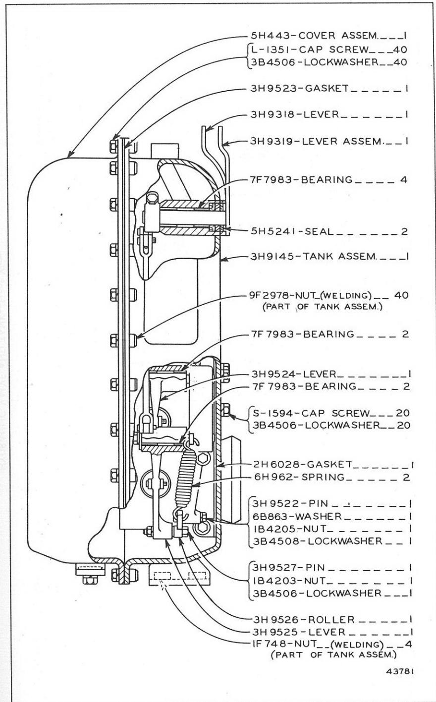
**HYDRAULIC VALVE AND TANK—End View**
