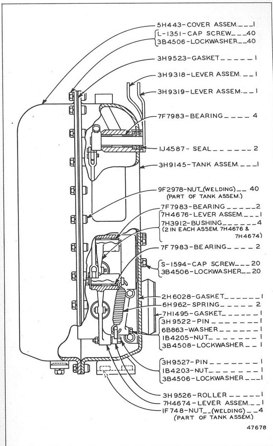
HYDRAULIC VALVE AND TANK—End View
