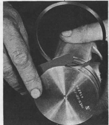
Fig. MH144—Checking piston ring side clearance.
