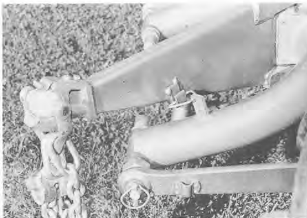
Fig. 33 - Coupler Boom in Locked Position
