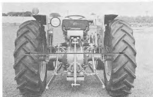
Fig. 42 - Rear Wheel Tread Width
