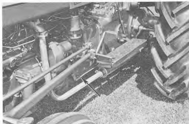
Fig. 78 - Brake Linkage Adjustment - Left Wheel
