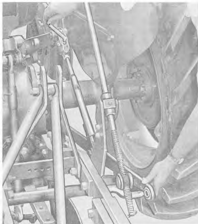
Fig. 27 - Attaching Right Lower Link to Implement
