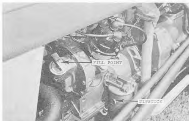
Fig. 13 - Crankcase Oil - Check and Fill Points
