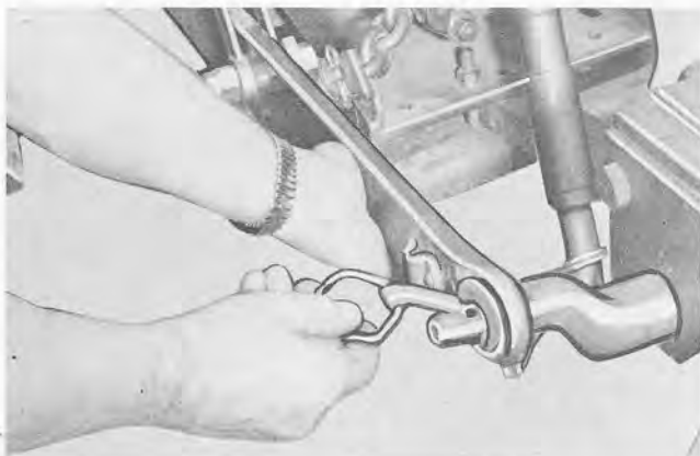
Fig. 26 - Attaching Left Lower Link to Implement
