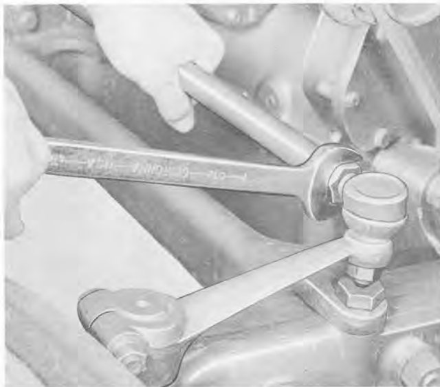
Fig. 80 - Adjusting Drag Links
