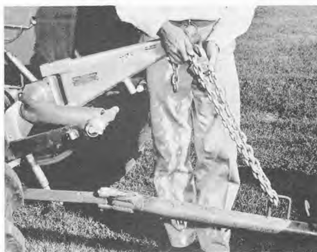
Fig. 30 - Installing Coupler Chain to Implement
