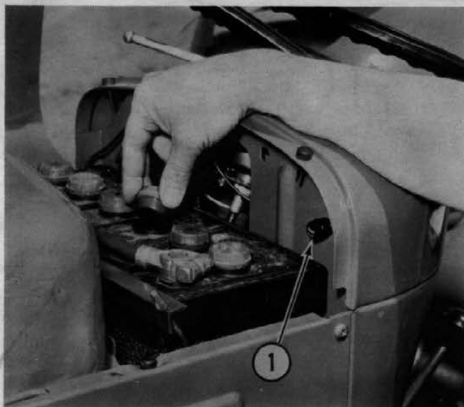
Checking Battery Water Level
