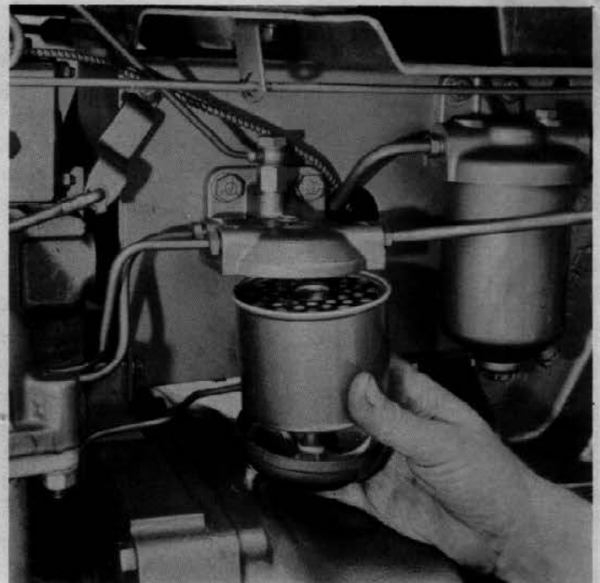
Servicing the Second Stage Filter
