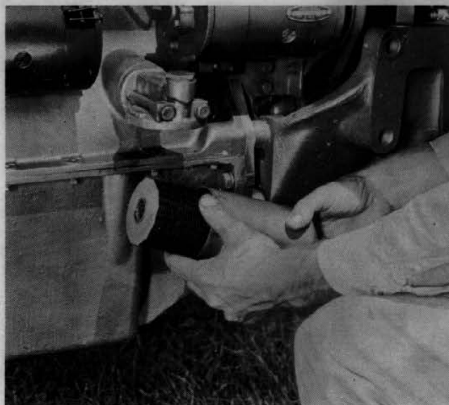
Removing Engine Oil Filter
