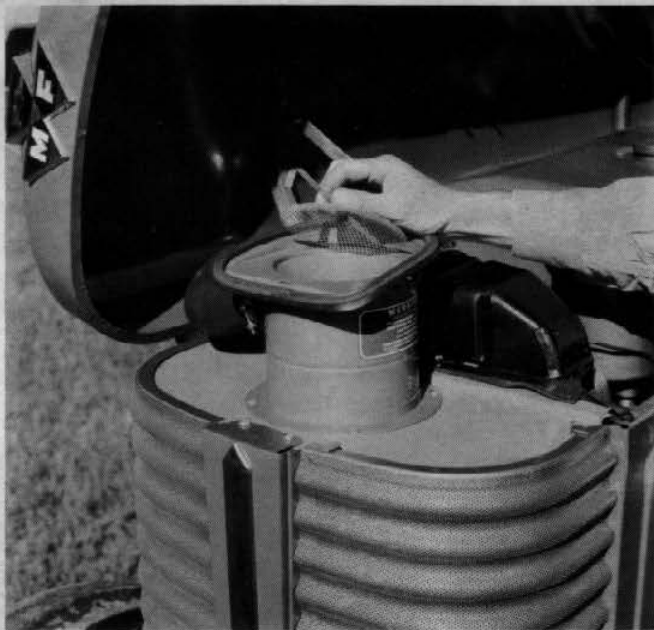
Removing Air Intake Screen
