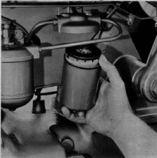
Servicing the First Stage Filter
