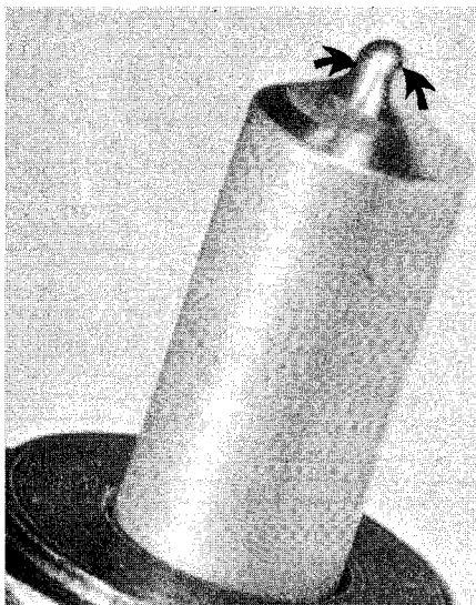
Fig. 88—Nozzle holes (arrows) are not located at equal distance from nozzle tip.
