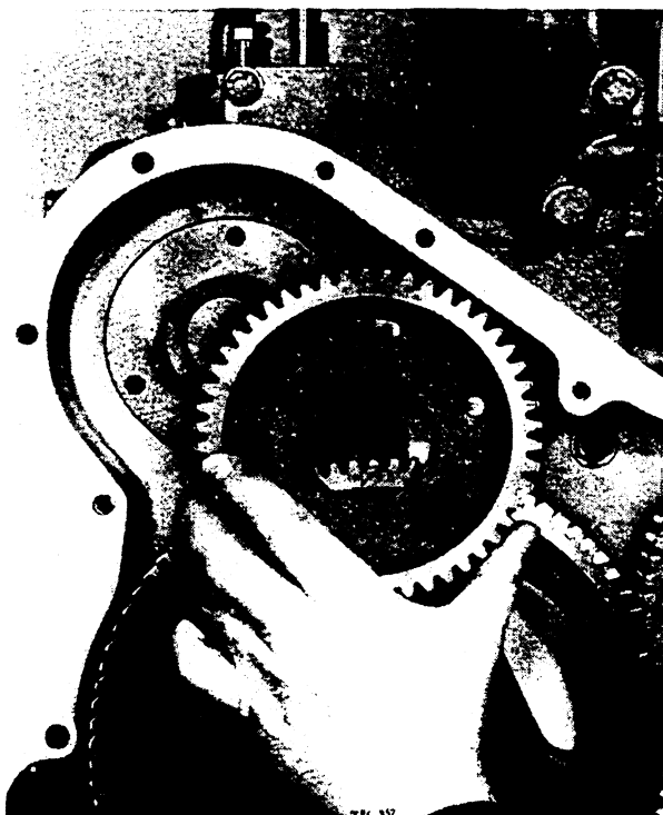
FIGURE 23 REMOVING CAMSHAFT GEAR
