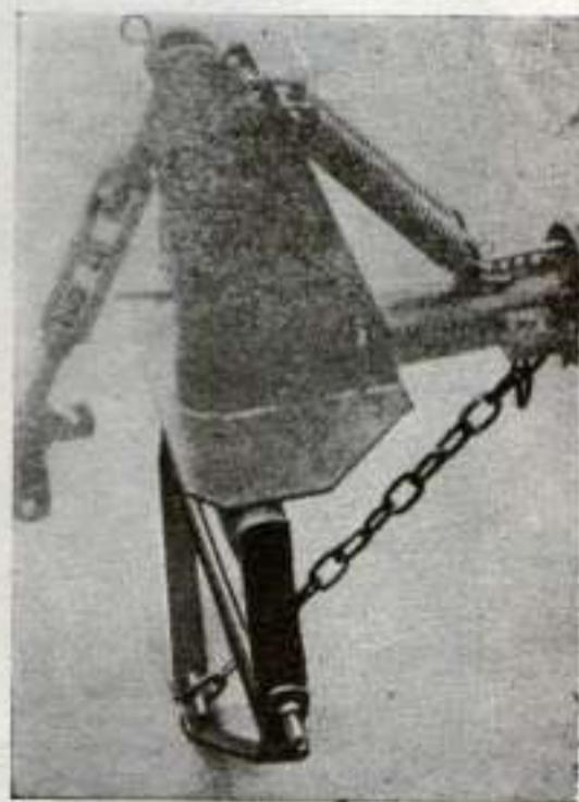
Fig. 11 - BEQUILLE PERMETTANT LA MISE AU REPOS DU RATEAU
