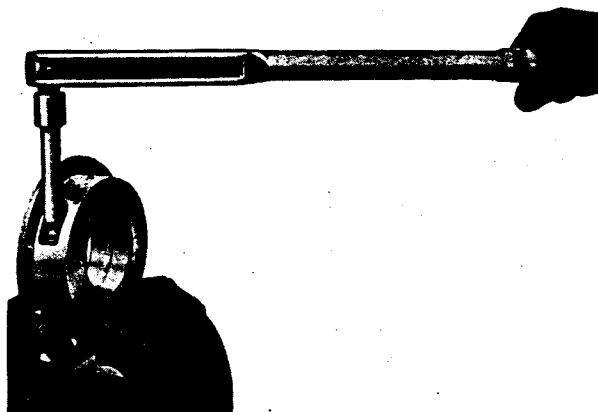
FIG. 155. TIGHTENING SOCKET SCREWS OF FRONT BEARING HOUSING USING SERVICE TOOL FT. 113 (OR FT. 86) WITH TORQUE WRENCH
