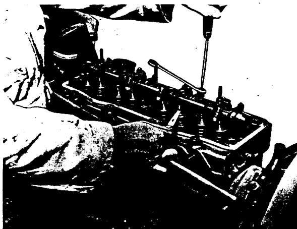
FIG. 111. ADJUSTING VALVE TIP CLEARANCES.
