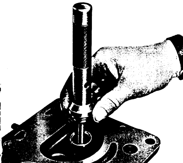
F.T.6057 VALVE SEAT INSERT REPLACER (TE-20 only) Replaces Valve Seat insert Part No. 1678
